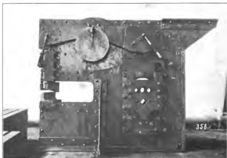
Fig. 4995. Johns Patent Bar Cutter Combined with Shear. Henry Pels & Co.
